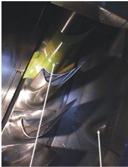
Rotor surface mounted pressure sensors Downstream vane leading edge
