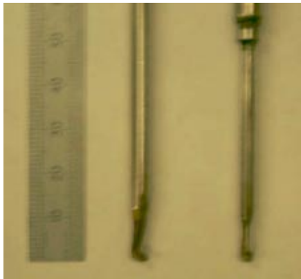
Fig. 2 Four-hole probe for low speed (left), current probe for high speed (right)
